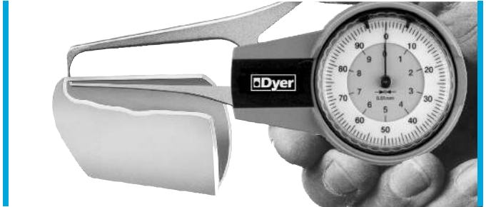
313 Special Model 313-405 modified to measure wall thickness of nozzle partition for turbine engines.
