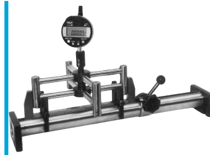
Model 440-202 Set Master with 440 Series Twin Cross® Bore Gage in a horizontal axis mastering setup.
