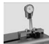
Adapter set up for groove gages
